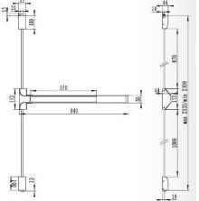
Touch bar vertical rod panic bolt with two point latching.
